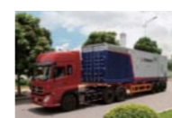
2011 Developed the MEGANINJA, a container-configured 1.5 MW gas engine power generation system that can begin generating power within 24 hours of delivery
