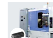
1997 Completed the world's first dry-cut gear cutting system, which uses no cutting oil
