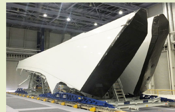
Composite material wing of a Boeing 787
