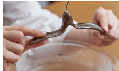
The shape-memory items made of polymer resin have handles that can bend into an easy-to-hold shape
