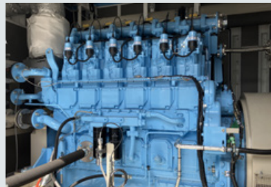
500 kW-class 6-cylinder hydrogen engine (prototype)
