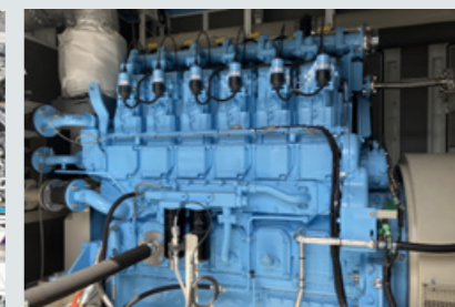
500 kW-class 6-cylinder hydrogen engine (prototype)
