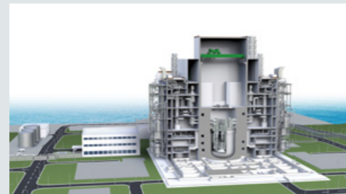
Sodium-cooled tank-based fast reactor (includes research results from projects commissioned by the Ministry of Economy, Trade and Industry)
