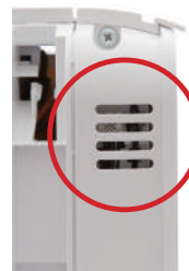
Sensor for indoor temperature and humidity
