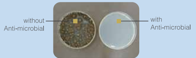
In tests conducted at the Mitsubishi Heavy Industries Nagoya Research Lab, 24 hrs after contact with bacteria, cultured on agar media.
