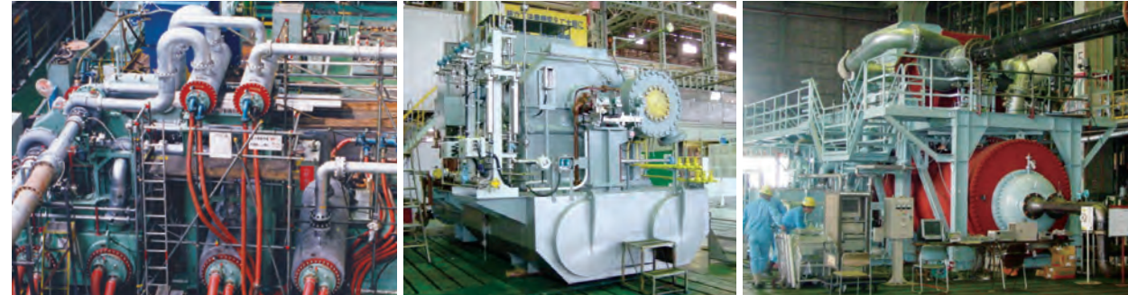
Nitrogen gas compressor (Combined type) for air separation plant
