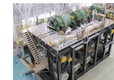
Nitrogen injection compressor module for ASU Plant
