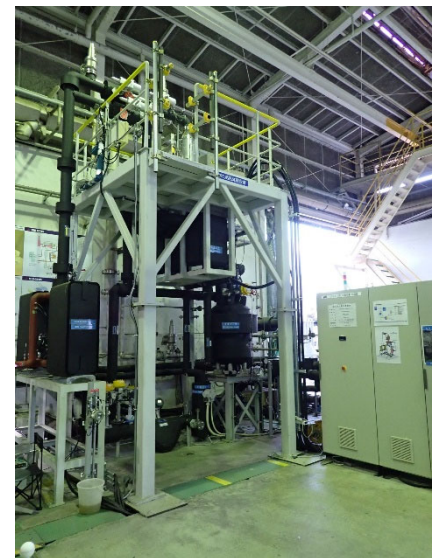
100kW class cryogenic ORC power generation demonstration testing equipment
