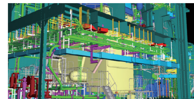
MATES® Machinery Room 3D Design
