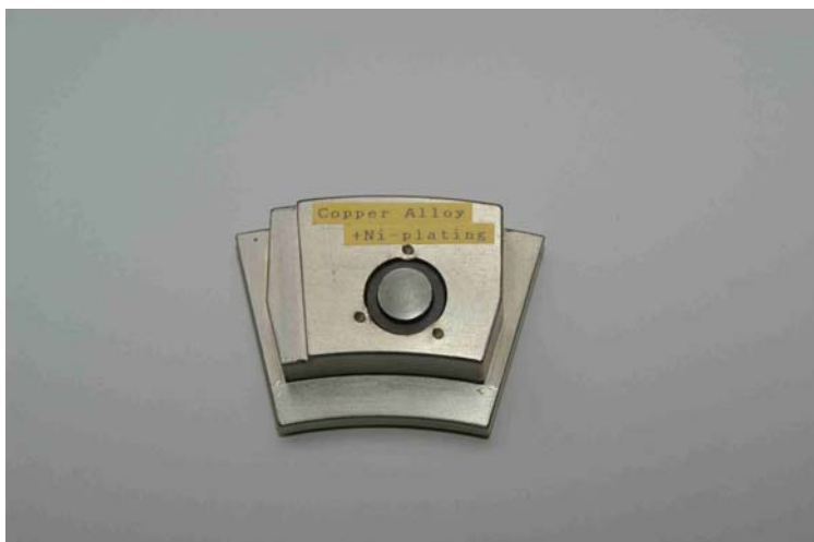
Thrust bearing pads (copper alloy back metal) with Ni-plating
