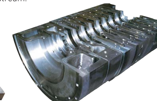
Diaphragm assembly for vertically split type
