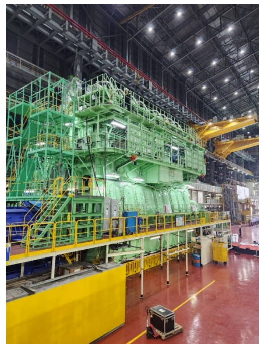
Dual-fuel methanol main engine equipped with a MET turbocharger (MAN ES 8G95ME-C10.5-LGIM)
