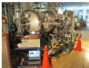
Fig. 12: Quenching test of the Main Accelerator Module
