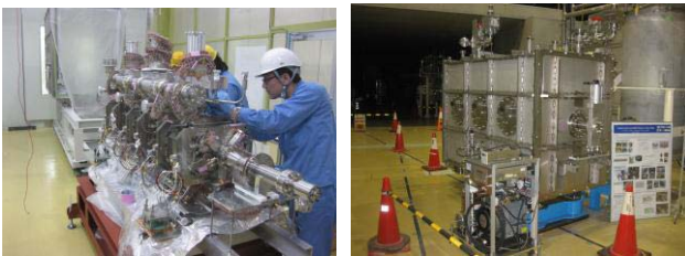
Fig. 6: Assembly and installation of the Injector Cryomodule (@ KEK-ERL Development Bldg.)
