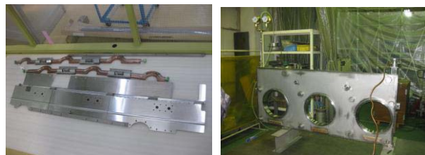
Fig. 3: Examples of component parts, (a) Thermal Shield and piping, (b) Helium Panel.
