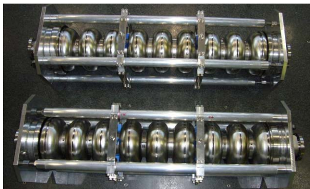
Figure 3: The STF 1.5-type cavities with transport jig
