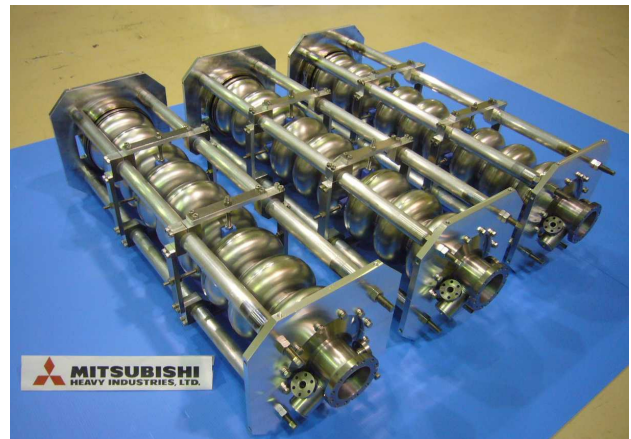
Figure 2: STF cavities governing the high-pressure gas safety law in Japan.
