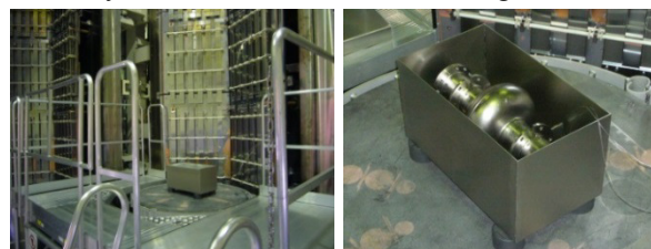
Figure 5: Heat treatment setup.
