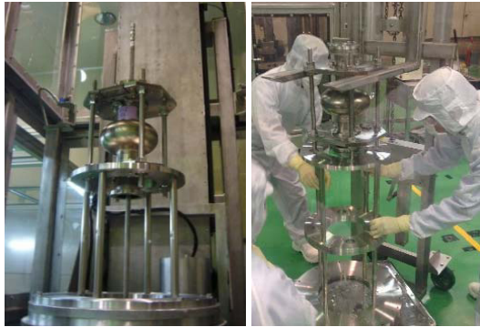
Figure 7: (left) HPR setup (right) Final assembly of the cavity.
