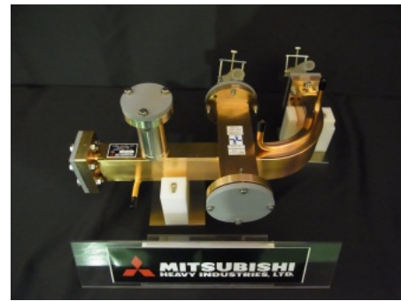
Figure 2: Completed E bend.
